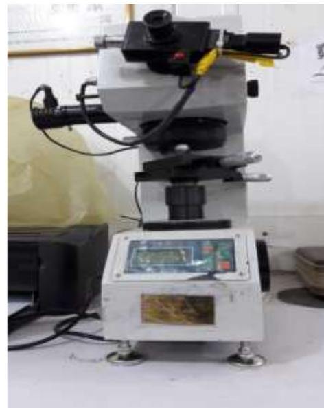
**Fig. 7;** Microhardness Tester
