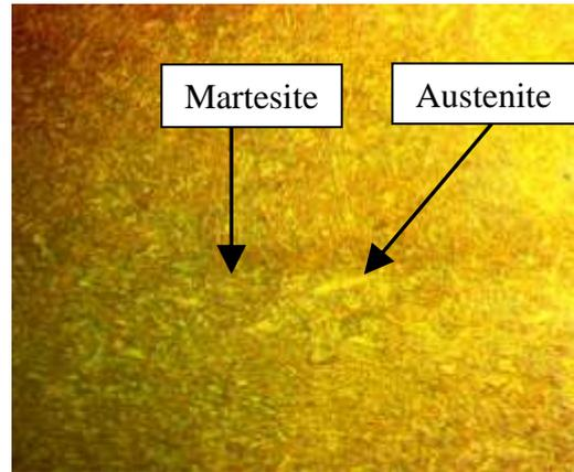
**Fig.11;** Water Tempering at 200°C with (80x)
