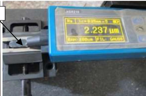
**Fig. 5;** Device of surface roughness test
