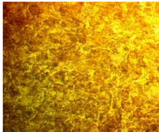
**Fig.15;** Polymer tempering at 200°C with (80x)
