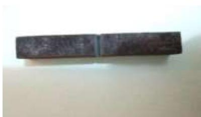
**Fig. 2;** Impact sample after heat treatment
