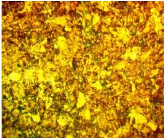
**Fig.14;** Polymer Quenching with (80x)
