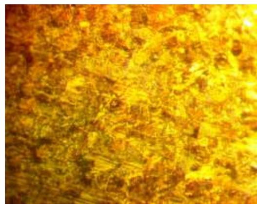
**Fig.19;** Oil tempering at 200°C with (80x)
