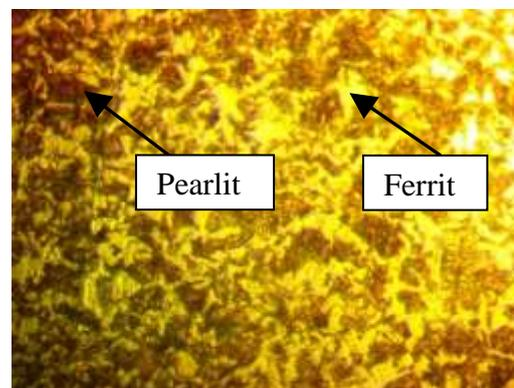
**Fig.9;** Microstructure with air cooling (80x)
