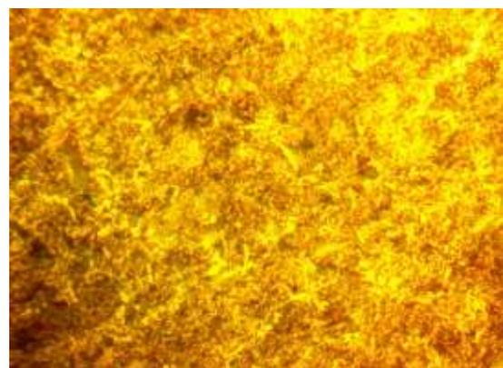
**Fig.21;** Oil tempering at 600°C with (80x)
