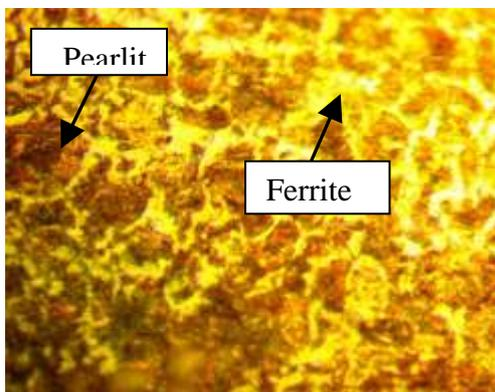
**Fig.8;** Microstructure of non-heat treated (80x)
