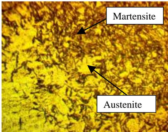
**Fig.10;** Water quenching with (80x)
