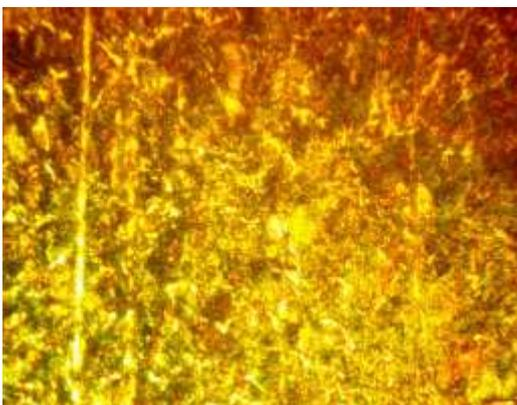
**Fig.20;** Oil tempering at 400°C with (80x)
