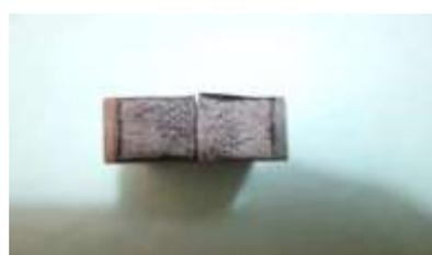
**Fig.3;** Sample after impact strength test
