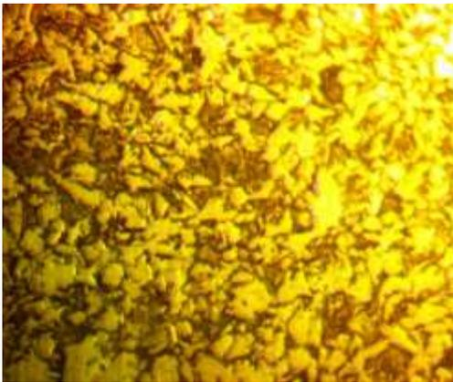
**Fig.18;** Oil quenching at (80x)
