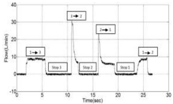
**Fig. (10):** flow curve at 2kg payload; floor level pattern (1→3→2→1→2)
