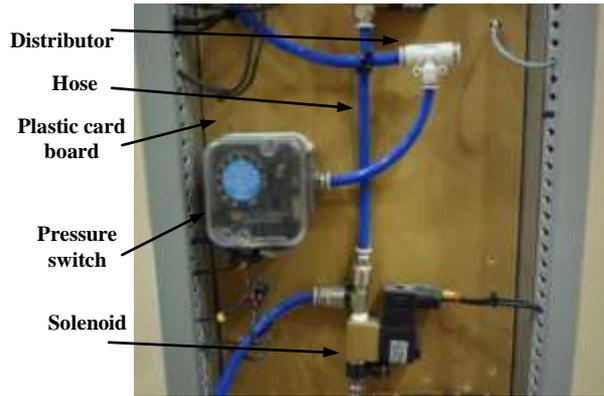
**Fig. (3) :** the back view; solenoid
