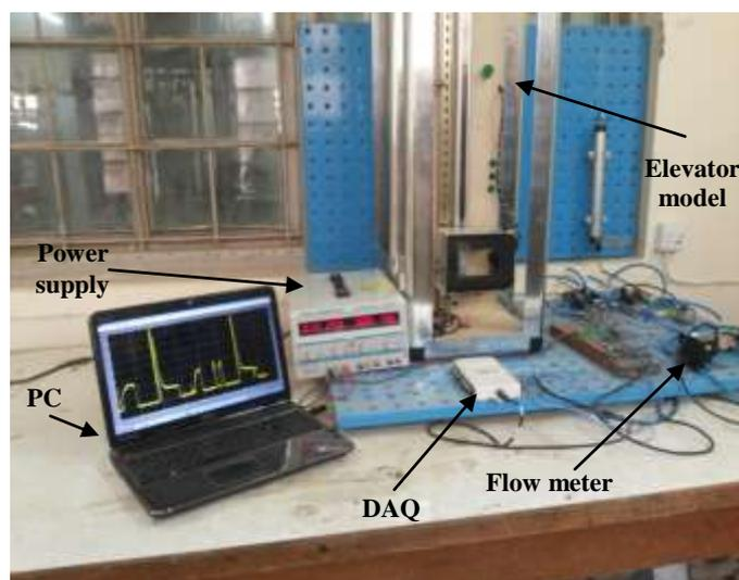
**Fig. (8):** the Experimental Setup
