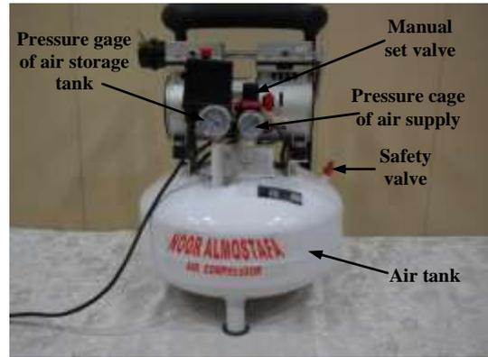
**Fig. (4) :** the air compressor
