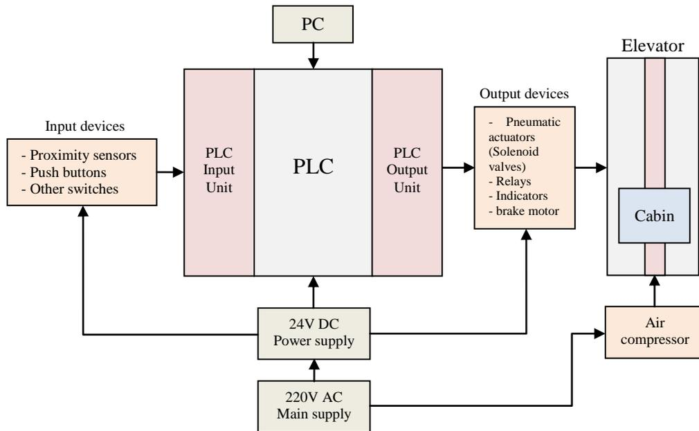
Fig. (1): Block diagram of the electro-pneumatic elevator
