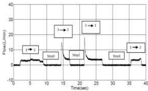
**Fig. (9):** No-load flow curve; floor level pattern (1→3→2→1→2)
