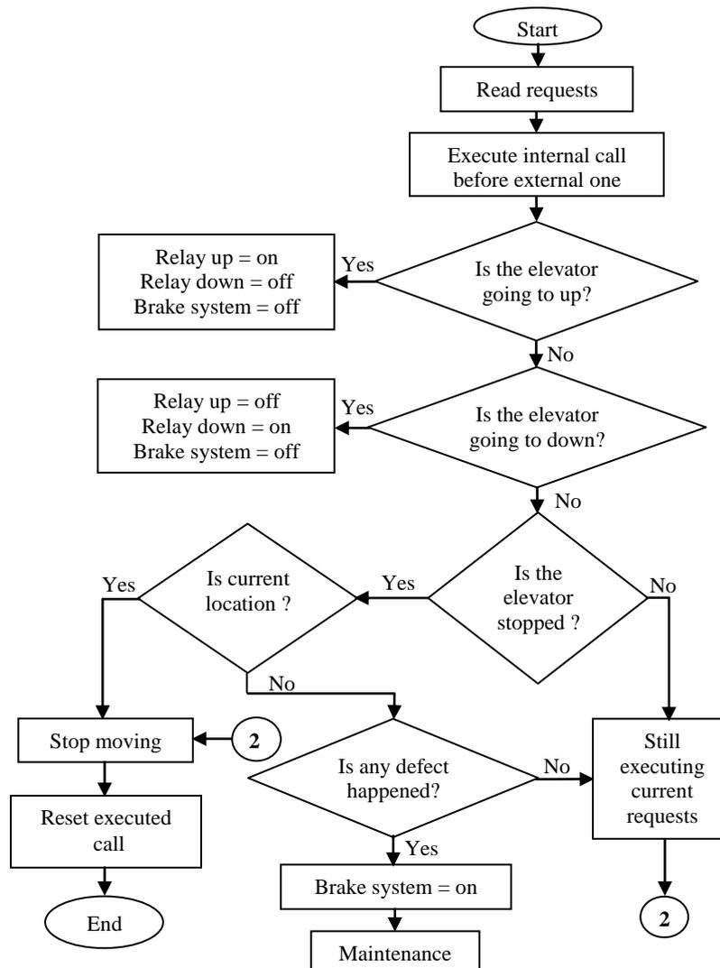
**Fig. (7):** Elevator control algorithm flowchart
