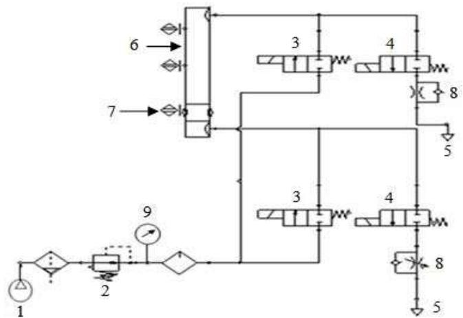
**Fig. (6):** Elevator Pneumatic Schematic Diagram
