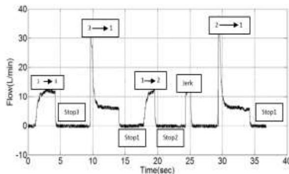
**Fig. (11) :** flow curve at 5kg payload, floor level pattern (1→3→1→2→1)
