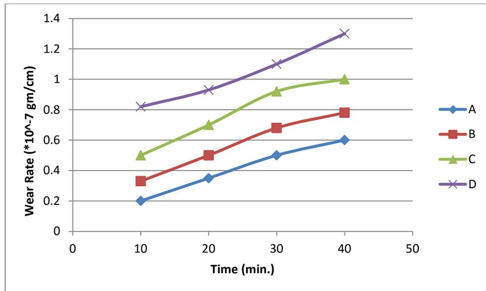
Figure (4): Relationship between Time and wear rate at constant load (1 kg) and sliding Speed (5m/s)
