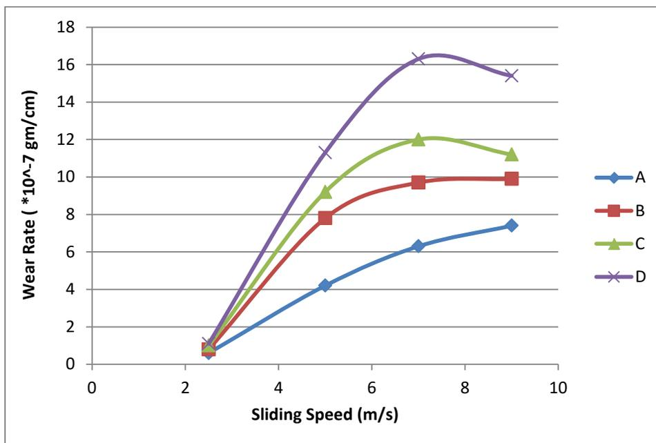
**Figure (6):** Relationship between ,Sliding Speed and wear rate at constant time (10)min and load (1 kg)
