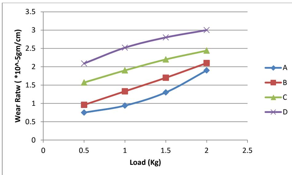
**Figure( 5):** Relationship between Load and wear rate at constant time(10)min and sliding speed of (5)m/s
