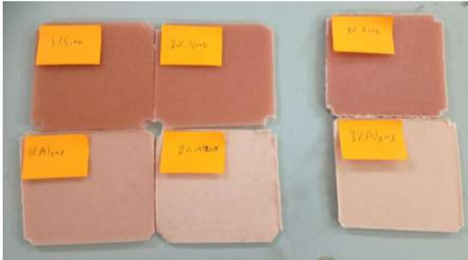
Fig. 3 Composite Prosthetic Dentures Specimens after Curing Process.
