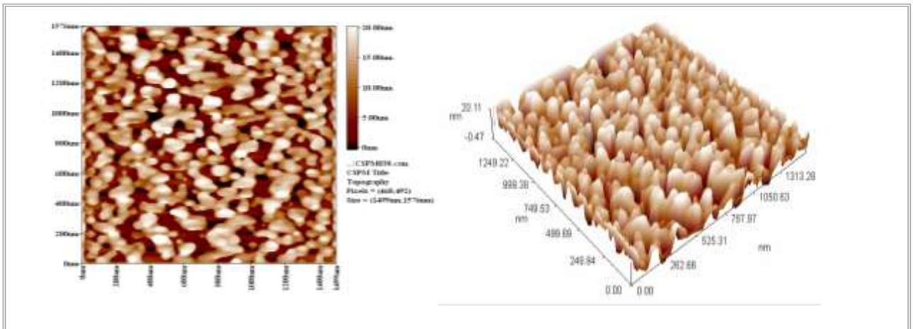
Fig. 1 AFM Test of Nano-SiO<sub>2</sub> Particles.
