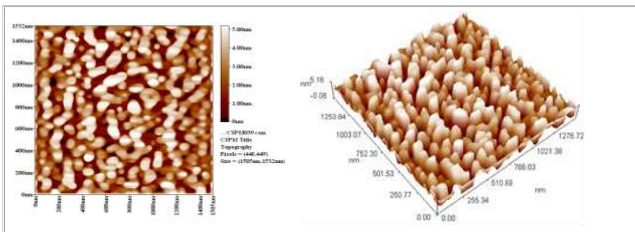
Fig. 2 AFM Test of Nano-Al<sub>2</sub>O<sub>3</sub> Particles.
