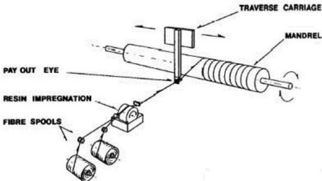
Fig (4) Schematic representation of the wet filament winding process
