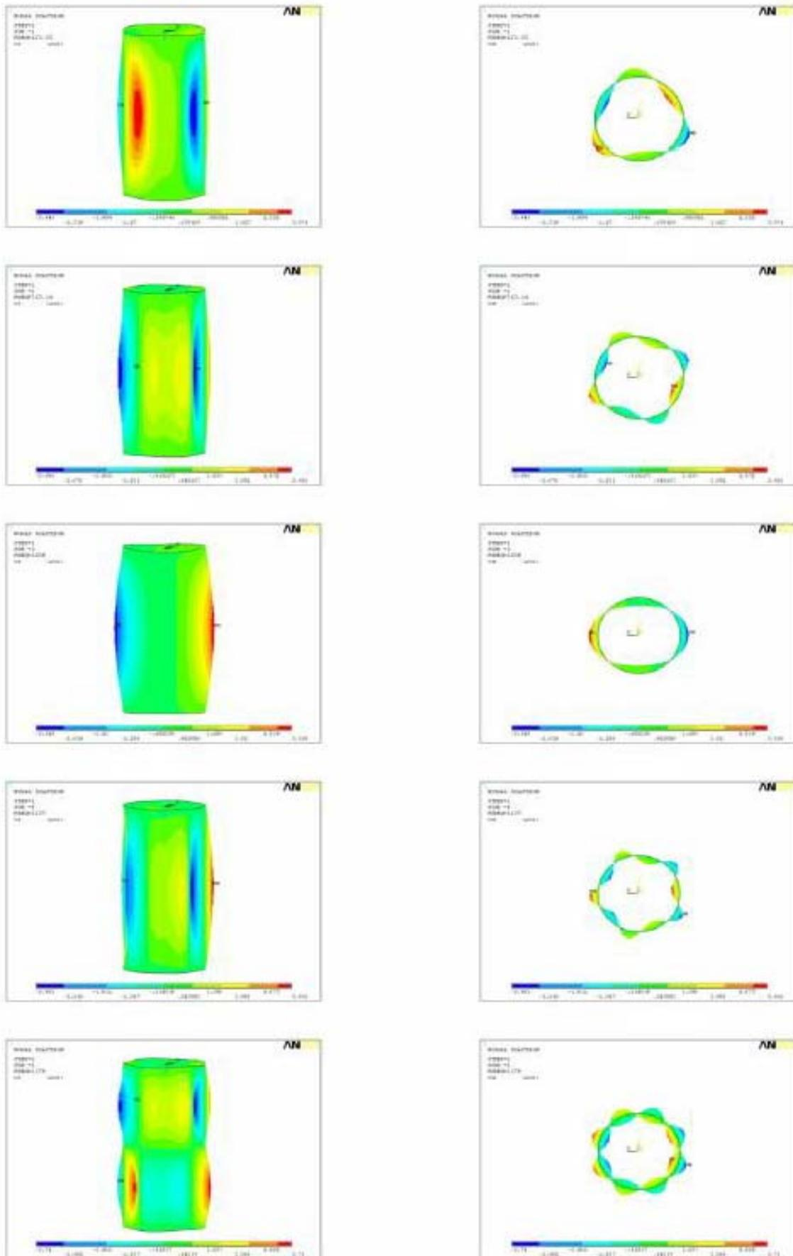
Fig.(7) Different mode shape of the cylinder under buckling condition
