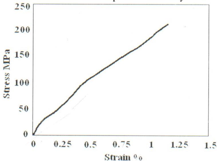
Figure (3) Tensile test results for Glass/ Polyester composite
