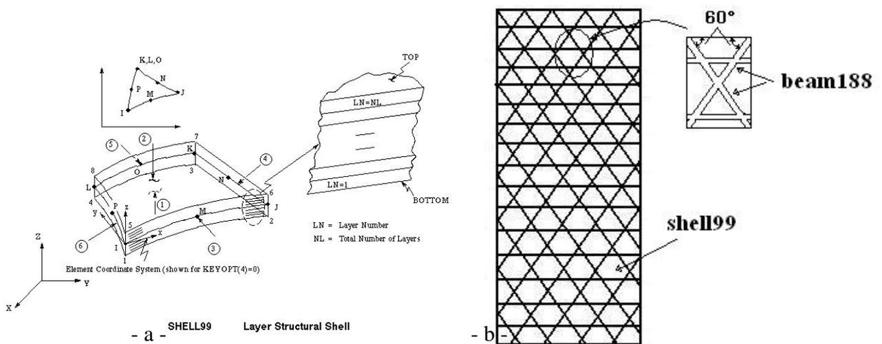
Fig.(2) a- Element shell99 b- Section of arrangement of the stiffeners
