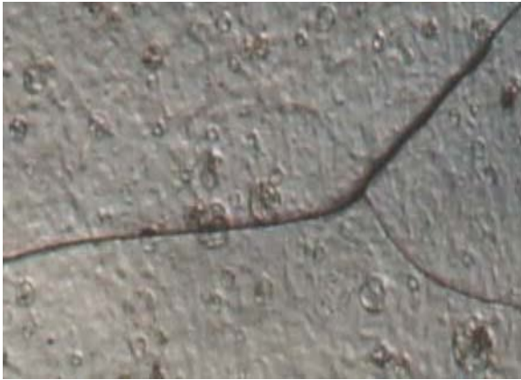
Figure 2-4 Some crake in \text{Al}_2\text{O}_3 film on glass substrate.
