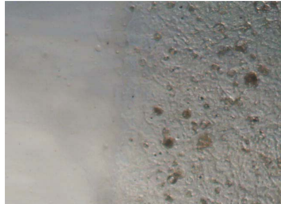
Figure 2-3 Interface of \text{Al}_2\text{O}_3 film on glass substrate
