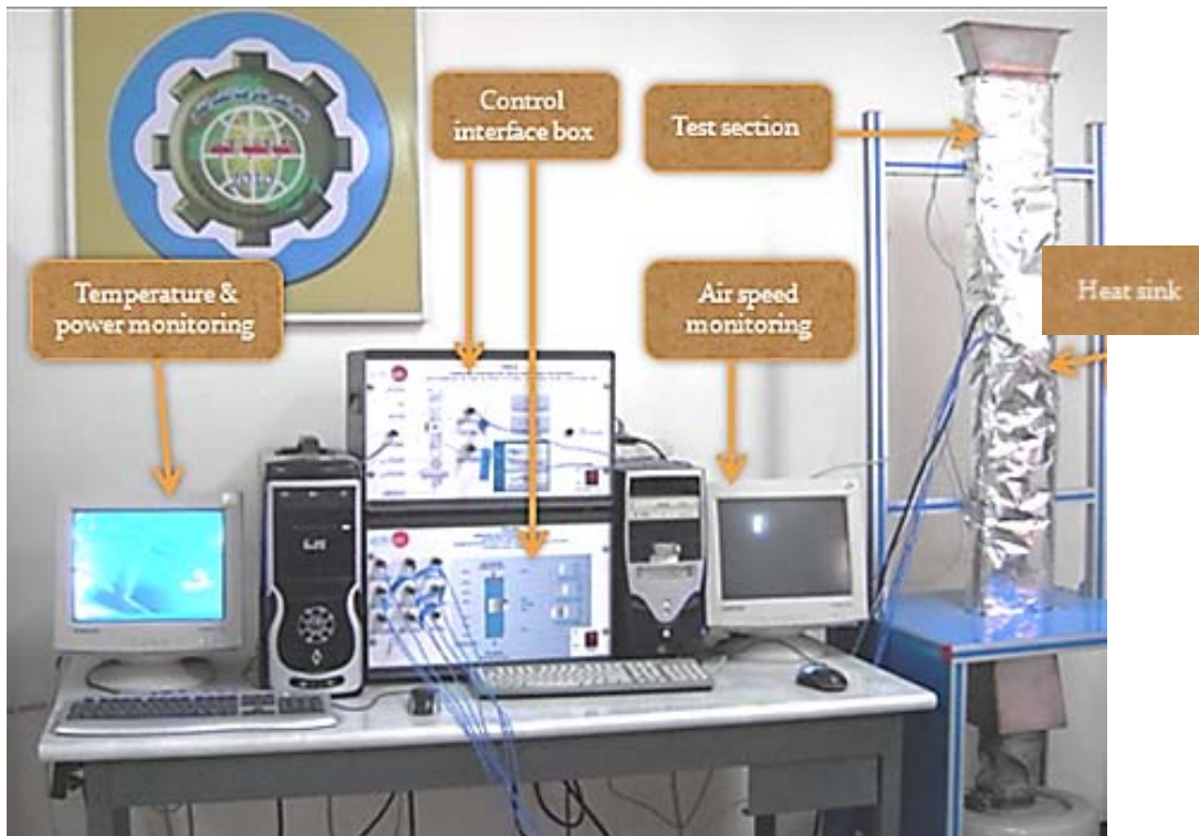
Fig. 1a: photographic diagram of the experimental rig.
