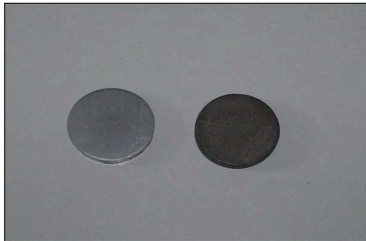
Figure (1): Austenitic stainless steel 316L alloy (a) as polished, and (b) as coated condition (chromized-siliconized diffusion coating specimen).
