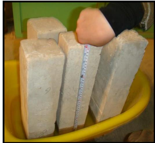
Fig (1) : Measure the water level of capillary rise
