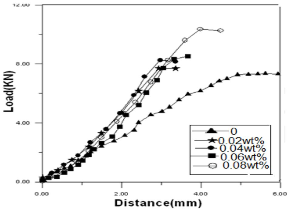
Fig.(7): data of compression test for epoxy specimens reinforced with PEG (0.02-0.08) wt %
