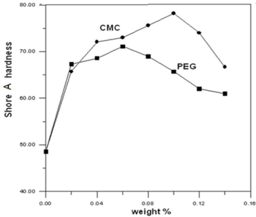
Fig. (2): Relationship between Shore A hardness and the weight fractions of CMC and PEG4000.
