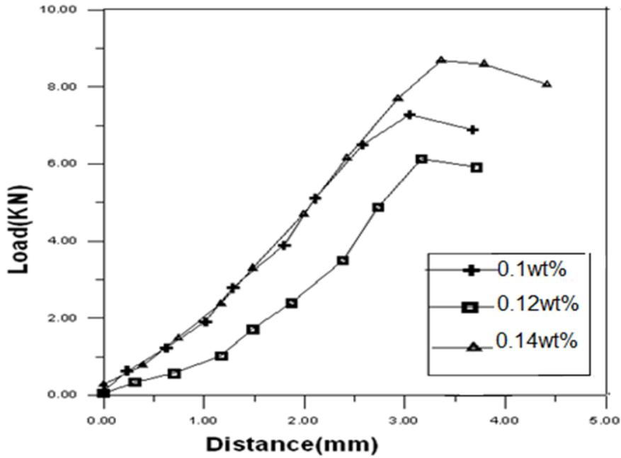
Fig.(8): data of compression test for epoxy specimens reinforced with PEG (0.1-0.14) wt %
