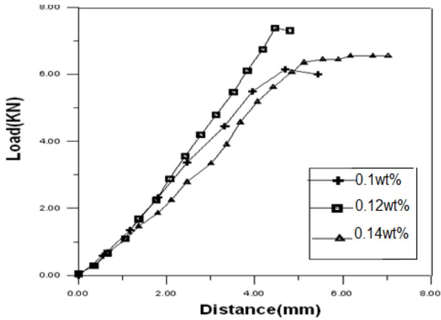
Fig.(4): Data of compression for epoxy specimens reinforced with CMC (0.1-0.14) wt %.
