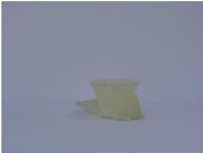
Fig.(5): Shape of failure of unreinforced epoxy specimen after compression test.
