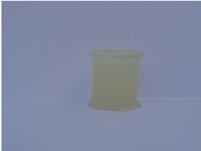
Fig.(6): Shape of failure of epoxy specimen reinforced with 0.12 wt % of CMC after compression test.
