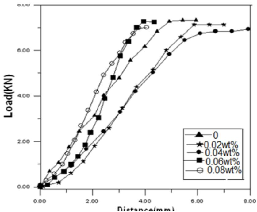
Fig.(3): Data of compression test for epoxy specimens reinforced with CMC (0.02-0.08) wt %.
