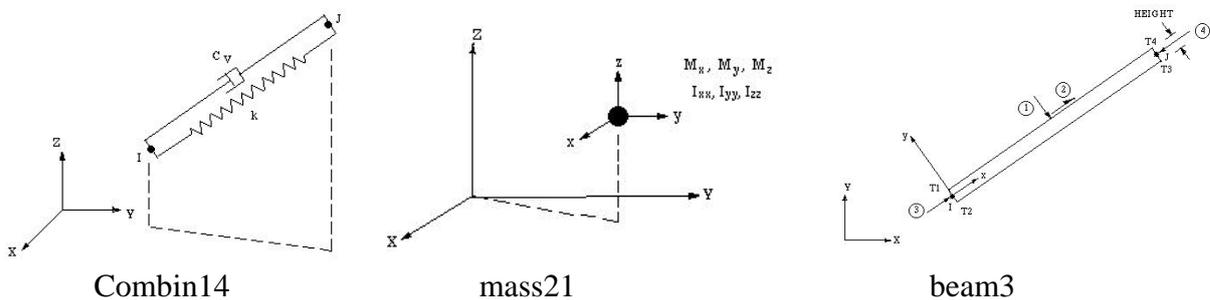
**Fig.9.** Elements used in the analysis
