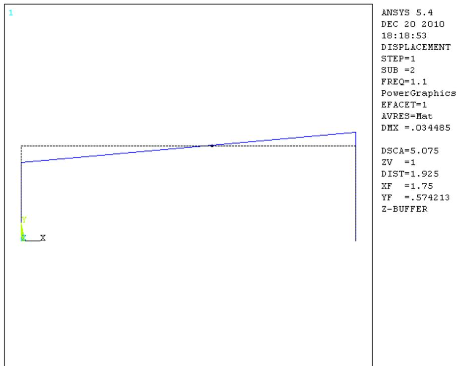
**Fig.12.** Mode shapes due to pitching effect
