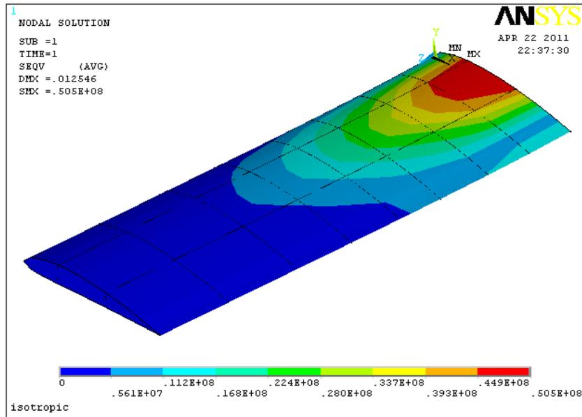
Fig.2 Von Mises stress distribution on the wing box.
