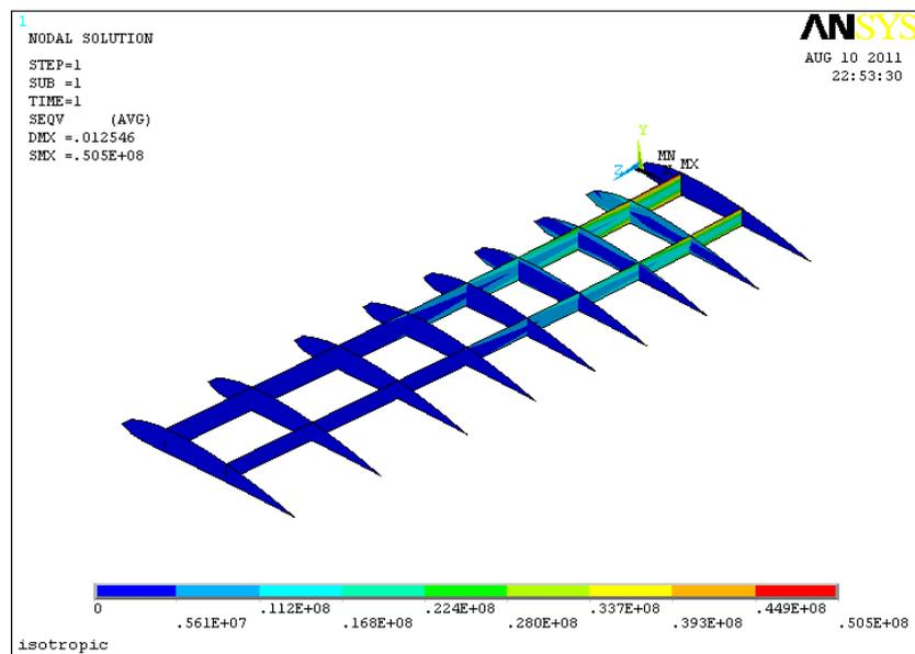
Fig.3 Von Mises stress distribution on internal structures of the wing box.
