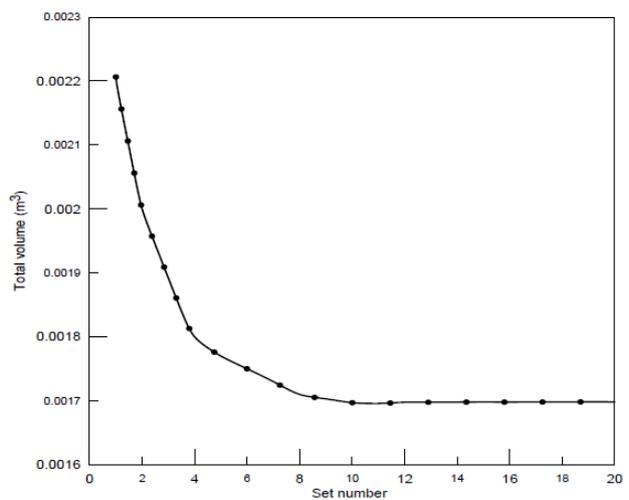
Fig.10 Total volume of the wing box versus set number.
