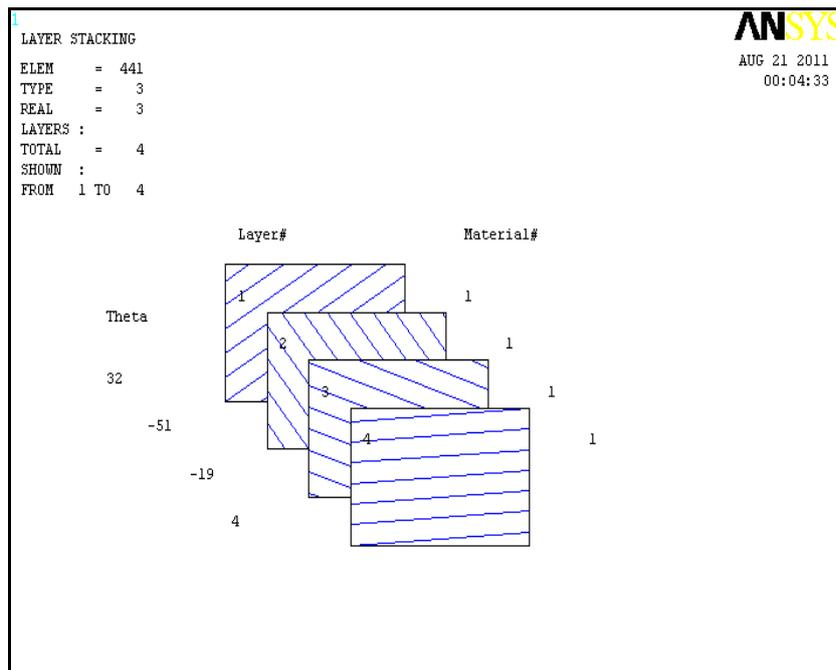
Fig.13 Optimum layers angles.
