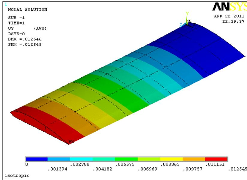
Fig.4 vertical displacement field-uy-on the wing box.
