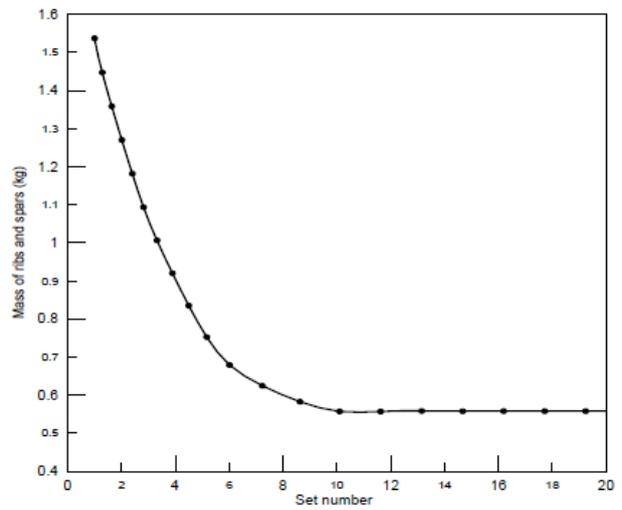
Fig.21 mass of ribs and spars versus set number.
