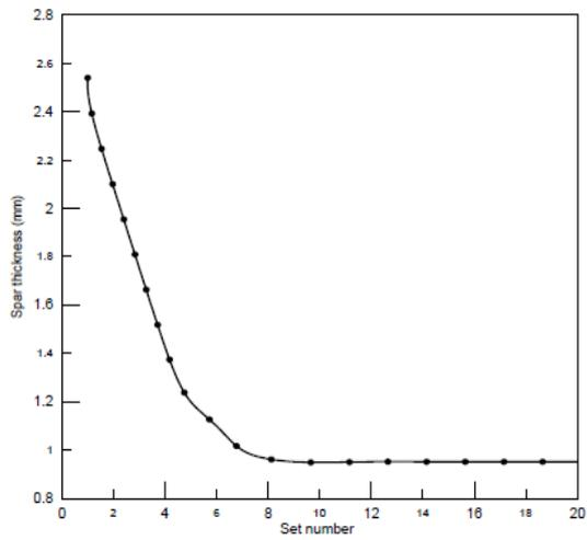
Fig.18 rib thickness versus set number.
