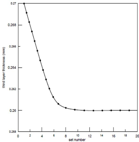
Fig.16 third layer thickness versus set number.
