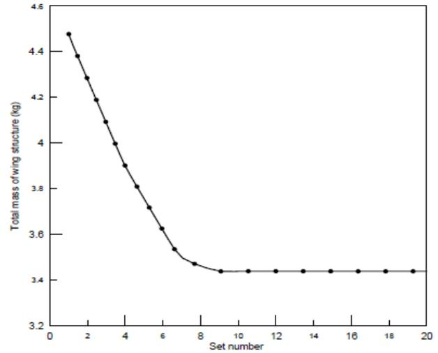
Fig.23 total mass of wing box versus set number.
